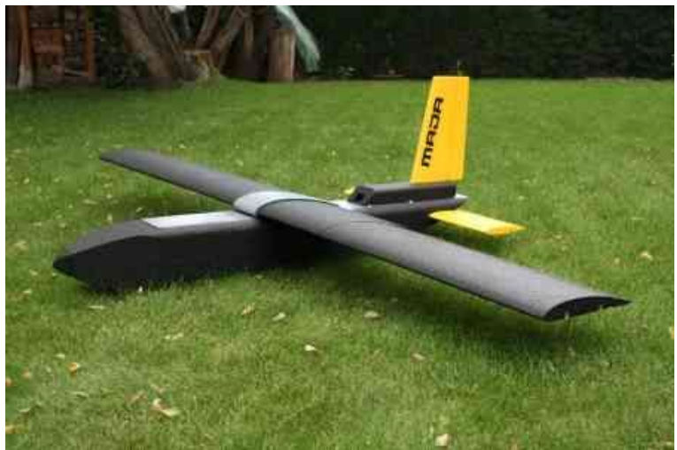
Figure 3: Fixed-wing drone—lightweight, more suitable for large areas
